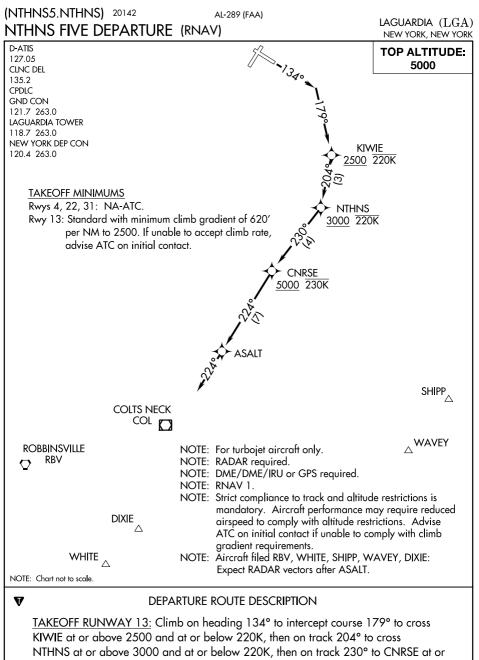
above 5000 and at or below 230K, then on depicted route to ASALT, then on track 224° for RADAR vector on course. Maintain 5000 or as assigned by ATC. Expect clearance to filed altitude/flight level 10 minutes after departure.
