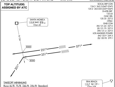
NOTE: TAKEOFF RWYS 24L/R, 25L/R: This departure is for non-turbojet aircraft. Turbojet aircraft use LAXX DEPARTURE. NOTE: South Complex turn at SMO R-154 to 201° is required for ATC separation.
