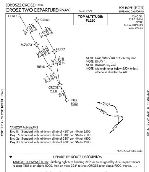
TAKEOFF RUNWAY 26: Climbing right turn heading 290° or as assigned by ATC, expect vectors to cross TILLR at or above 8000, then on track 324° to cross OROSZ at or above 9000, thence. . . .
