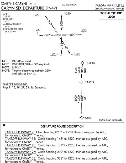
TAKEOFF RUNWAY 36: Climb heading 001° to 1220, then as assigned by ATC, for vectors to CMSKY. Thence....
