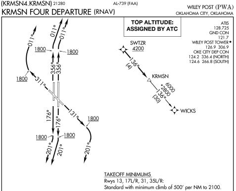
NOTE: RADAR required. NOTE: DME/DME/IRU or GPS required. NOTE: RNAV 1.
