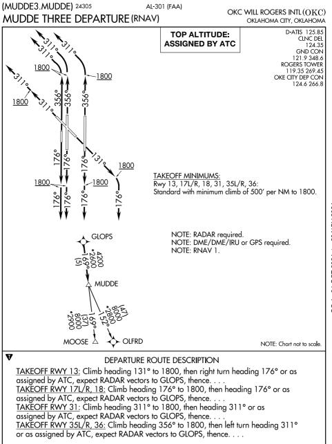
....on track 169° to MUDDE, then on (transition). Maintain 5000 or as assigned by ATC. Expect filed altitude 10 minutes after departure.
