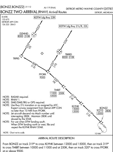
LANDING RWYS 22L. 21L/R: From FFORK on track 037° to cross TBRRD at 8000 and at 210K, then on track 036°. Expect RADAR vectors to final apporach course. LANDING RWY 22R: From FFORK on track 308° to TRPRS, then on track 035° to cross DZMND at 8000 and at 210K, then on track 033°. Expect RADAR vectors to final approach course.
