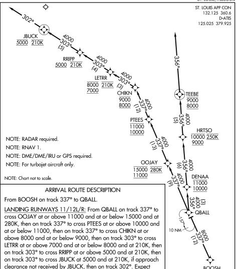
LANDING RUNWAYS 29/30L/R: From QBALL on track 356° to cross DENAA at or above 10000 and at or below 11000, then on track 356° to cross HRTSO at or above 9000 and at or below 10000 and at 250K, then on track 356° to cross TEEBE at or above 8000 and at or below 9000, then via assigned instrument approach procedure. If approach clearance not received by TEEBE, then on track 356°, expect RADAR vectors to final approach course.
