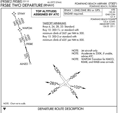
TAKEOFF RUNWAY 6: Climb on heading 060° or as assigned by ATC for RADAR vectors to ALNZO, thence....
