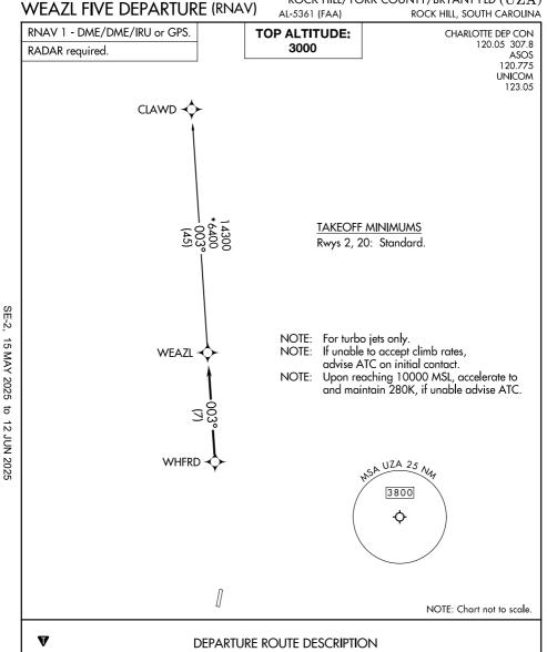
Climb on heading assigned by ATC, on RADAR vectors to WHFRD, then on track 003° to WEAZL. Then on CLAWD Transition. Maintain 3000, expect clearance to filed altitude within 10 minutes after departure.
